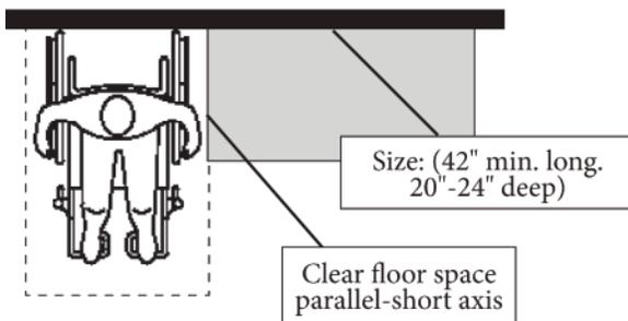
Providing the clear floor space at the end of the bench as required by the 2010 Standards instead of in front of the bench as is allowed by the 1991 Standards would only be required when the bench in the accessible dressing room is altered or when the entire dressing room area is altered.
